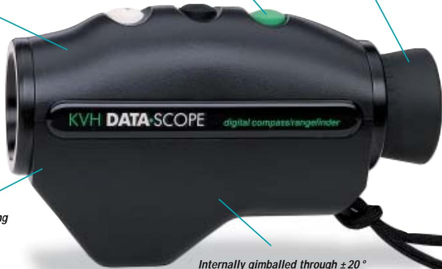
**Internally gimballed through  $\pm 20^\circ$**  so you don't have to hold it perfectly level and steady for 0.5° accuracy.
