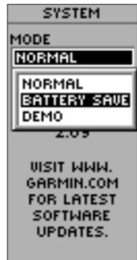
*The eTrex's batteries will last up to 22 hours in 'BATTERY SAVE' mode (when using alkaline batteries).*
