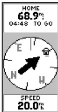
The arrow tells you what direction you should move. When the arrow is pointing right as shown here, just move right until the arrow is pointing straight up and points to the moving direction line (see picture below).
