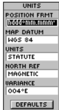
*The 'UNITS' Page allows you to match the units of the eTrex to the units of a unique paper map you may be using.*
