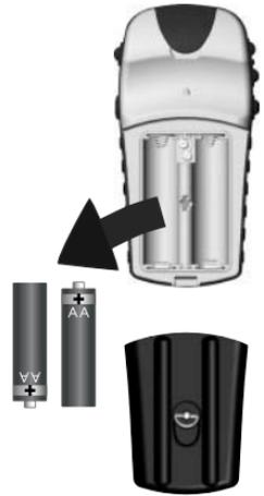
*Remove the batteries from your eTrex if you don't expect to use it for several months. Be sure to observe the proper polarity when re-installing batteries. Follow the battery manufacturer's instructions on the proper care and handling of the batteries.*
