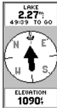
*The Navigation Page allows you to display eleven types of different data, such as ‘Elevation’.*
