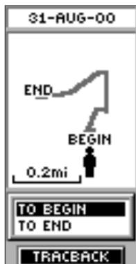
The 'BEGIN' point is the point defining the starting point when saving a track log. 'END' is the last point that was saved. Each saved track will always have a 'BEGIN' and 'END' point for navigation. The 'BEGIN-END' pair imply the direction of the saved track. If you want to retrace the track, navigate to 'END'. If you want to track back to the starting point, navigate to 'BEGIN'.
