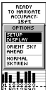
Pressing ENTER on the Advanced Skyview Page also offers the options of Orienting the Sky Ahead or Northward, Setup Display (backlighting/contrast), and returning to Normal Skyview.
