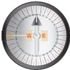
The *eTrex* is not a magnetic compass. You must be moving in order for it to track your movement.
