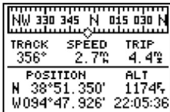
The screenshot shows a GPS display with a graphic compass at the top. Below the compass, the text reads: TRACK 356°, SPEED 2.7%, TRIP 4.4%. At the bottom, it shows POSITION: N 38°51.350', W 094°47.926', ALT 11745, and a time of 22:05:36.
