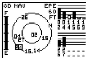
Check the Satellite Page for '2D nav' or '3D nav' to verify a position fix.
