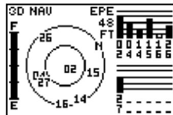
*The signal strength bars give you an indication of what satellites are visible to the receiver, whether or not they're being used to calculate a position fix, and the signal quality.*
