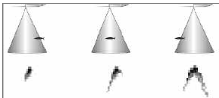
Transducer Cone and Fish Arches
