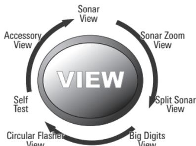
The sonar information from your Fishfinder is displayed on the screen in a variety of easy-to-read views. There are many views available on your Fishfinder. When you press the VIEW key, the display cycles through the available views on your screen. When you press the EXIT key, the display cycles through the available views in reverse order.
