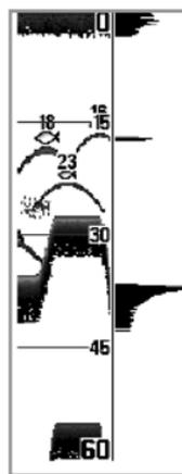
The **Wide RTS Window™** indicates the sonar intensity through the use of a bar graph. The length of the plotted return indicates whether the return is weak or strong. The depth of the sonar return is indicated by the vertical placement of the return on the display depth scale. The Wide RTS Window™ does not use grayscale.
