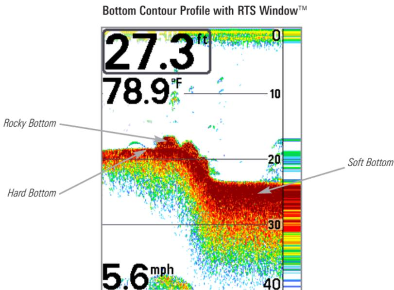
The sonar returns from the bottom, structure, and fish can be represented as **WhiteLine™** or **Structure ID®**. See *Sonar Menu Tab: Bottom View* to set the bottom view.
