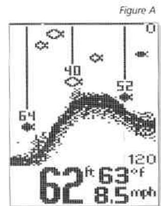
**Temperature/Speed.** The initial screen layout takes one of two basic forms depending on whether the optional Temp/Speed accessory is installed. Figure A shows the default view when the Temp/Speed accessory is installed. Figure B shows the default view when the Temp/Speed accessory is not installed.
