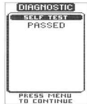
**Self Test.** Initially the 200DX will perform a self-test. This test confirms the operation of all internal circuitry. At the conclusion of the test one of two messages will appear. "Passed" indicates the internal test discovered no failures, "Failed" indicates a significant internal problem was discovered and the unit requires factory service. A code number appears that tells repair personnel where the problem is.
