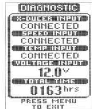
**Voltage Input.** Another connection tested is the voltage input, and is especially helpful in diagnosing input voltage problems. The current input voltage is displayed. If voltage fluctuations or power supply in excess of 20 VDC or less than 10 VDC is suspected, use the diagnostic screen to confirm input voltage. Often small outboard motors do not effectively regulate voltage when operated at high engine speeds.
