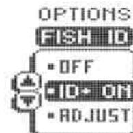
ID+ On enables the 200DX to interpret the raw sonar data, and using a variety of techniques, depict appropriate target returns as one of three different size fish symbols. Further identification shows whether the fish is in the wide or narrow beam. The 200DX also displays the depth beneath the surface with the corresponding fish symbol.
