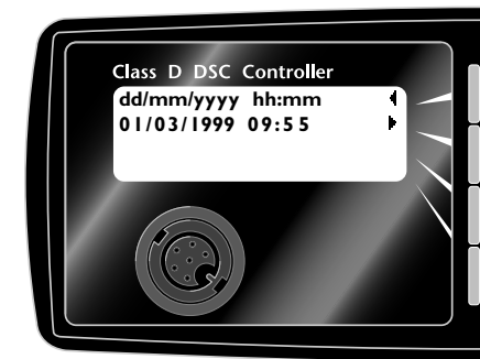
Fig 4.7 - Manually entering date & time
