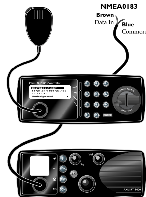
Fig 5.2 - Connecting DSC1400 to RT1400 + NMEA
