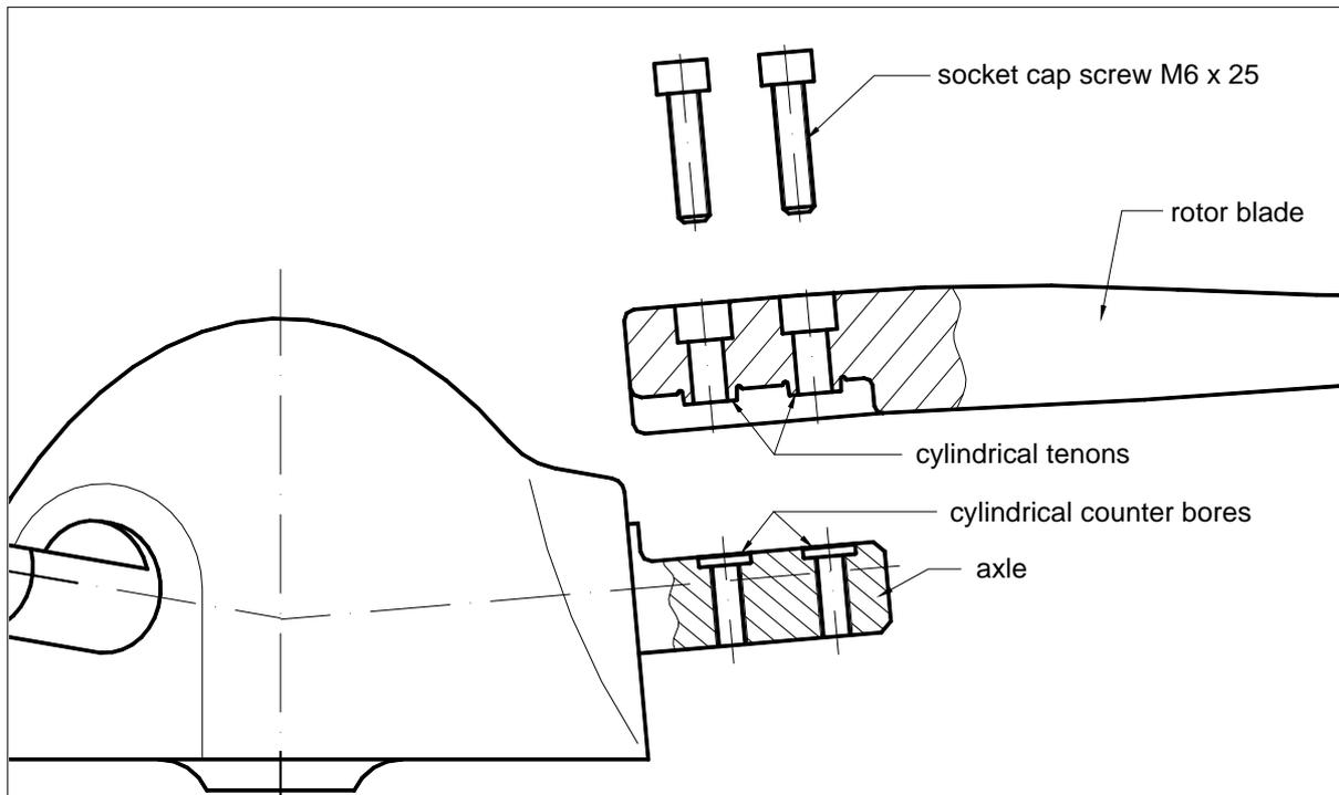
The rotor blades are fixed by two socket cap screws M6 x 25, which are TUFLOK-coated to prevent loosening at operation. When screwing in you will sense a slight drag torque due to the coating.
