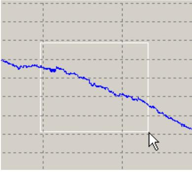
You can increase a cut-out of the air pressure curve. Draw in addition a rectangular window with the mouse from above left downward right. Use the left mouse button. If the mouse button is released, the appropriate range of the diagram will be shown increased.
