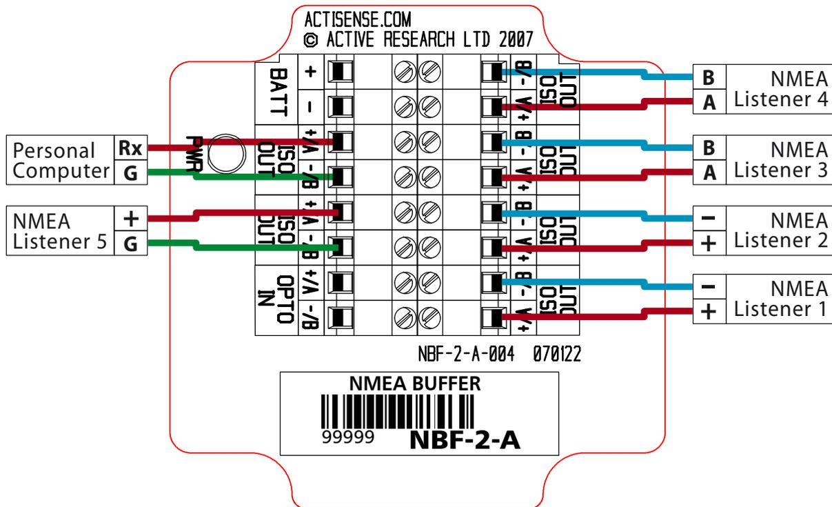
Figure 3 – Output connections
