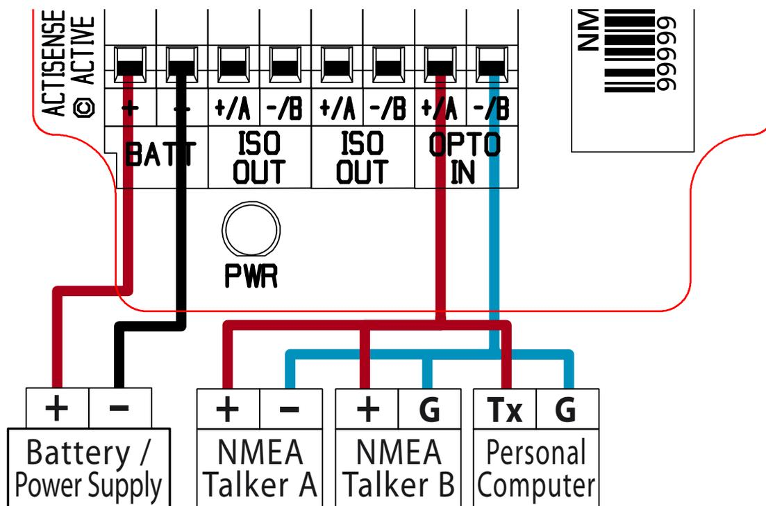
Figure 2 – Input connections
