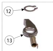
DETAIL, PAWL MOUNTING DIRECTION.
