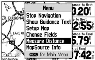
Use the 'Measure Distance' option to measure distance and bearing between any two map locations. A pointer and "rubber-band" will appear, along with display of bearing and distance between points at the top of the page.
