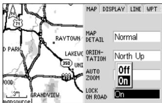
*'Lock On Road' causes the triangular present location symbol to "snap to" the nearest road. This compensates for any minor errors in your location reading.*
