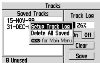
From the Saved Tracks Page, press **MENU** to select 'Setup Track Log' and modify the track log recording settings.
