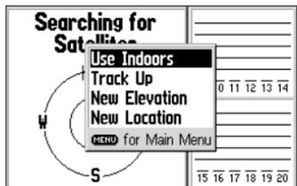
Select 'Use Indoors' to activate the built-in simulator mode. Do NOT attempt to use the GPS V for actual navigation while in simulator mode.
