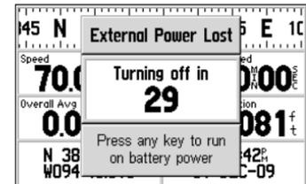
When external power is removed, the GPS V will alert you with a screen prompt. Press any key to continue operating the GPS V.
