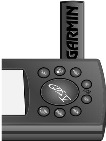
**POWER (Red Bulb Symbol)**- Turns the unit on and off. A momentary press while the power is on displays the backlight/contrast adjustment window. Press and hold to turn the GPS V off.
