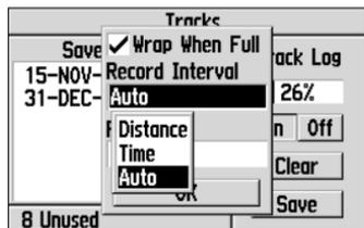
Track logs can be recorded by time, distance or 'Auto' intervals. 'Auto' uses a resolution function where additional track points are not saved until you deviate left/right from a projected course.
