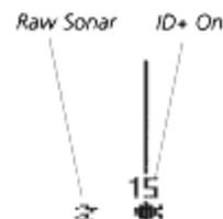
Increasing the value to a number greater than zero shows more fish symbols on-screen. In this case smaller sonar returns will be depicted as fish symbols. This is useful for identifying many smaller sonar returns (such as baitfish) as fish symbols.
