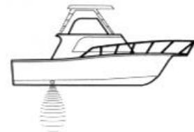
Thru-hull mounting may require the use of a fairing block to level the transducer with the waterline. Also, since special tools and knowledge may be required to perform this type of installation, it is best to refer to a qualified marine technician.
