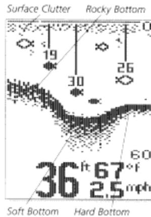
Wave action also affects the bottom depiction. The information drawn is a distance measurement, so if the boat is moving up and down over flat bottom, the bottom depiction often appears in regular variations that match wave timing.
