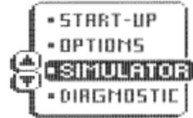
There are two ways to start the simulator. If the unit is powered off, press and hold the POWER button for approximately three seconds until you hear a continuous chirp.
