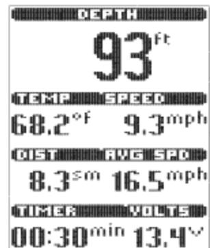
The time, speed and distance calculations are useful for tracking your progress on a trip. The input voltage is useful for determining the condition of the charging system of the boat. When used in a portable application or whenever the 300TX is operated from a battery source, the voltage number can be used to determine battery life. The 300TX will operate at voltages from 10 to 20 VDC. Voltages in excess of 20 or less than 10 VDC cause the unit to power off.
