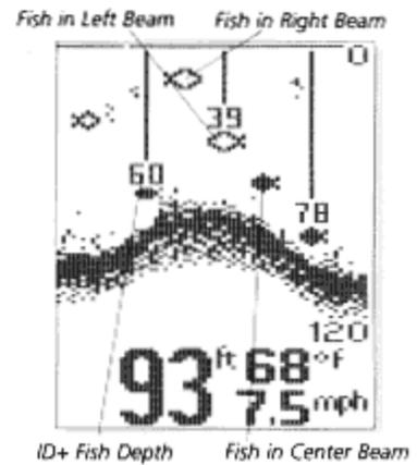
The specific fish symbol indicates the type of sonar beam the fish is detected in. This gives you a reliable indicator of side to side location relative to boat movement. Fish symbols which are hollow are detected in the outside two beams. Hollow fish symbols facing to the left are detected in the left beam, and thus the fish is to the left side of the boat. Solid fish symbols represent fish in the single center beam, and these fish are directly under the boat.
