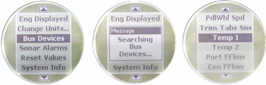
Bus Devices highlighted in the System Setup menu (left). Searching Bus Devices window (center) with Bus Devices list (right).
