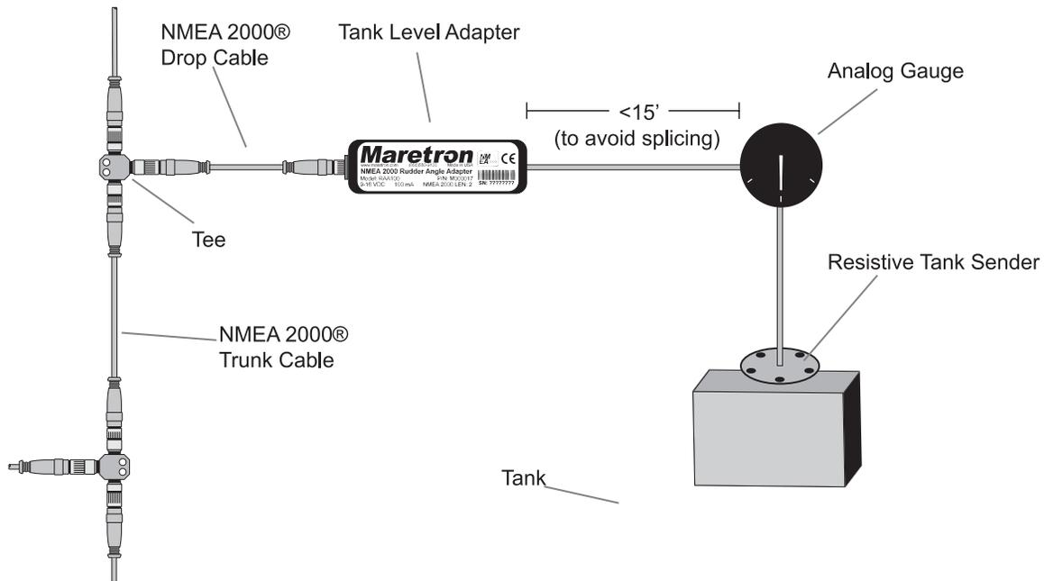
**Figure 1– Mounting Location When Used with Analog Gauge**
