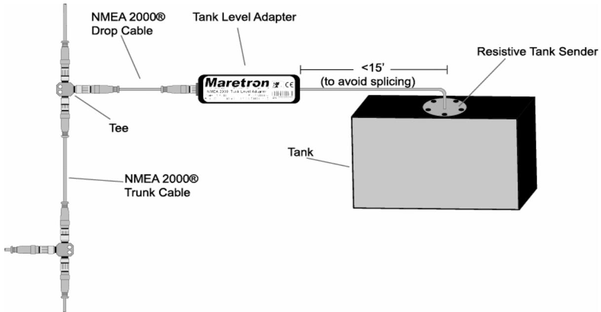
Figure 2 – Mounting Location When Used Without Analog Gauge
