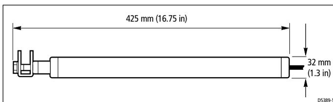
Linear rudder position sensor – dimensions
