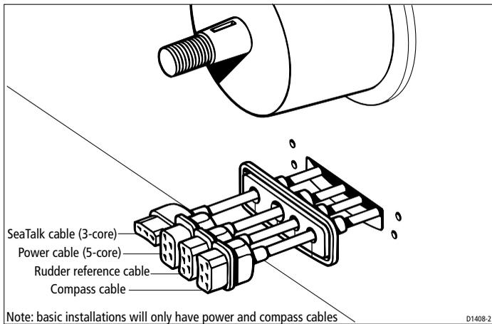
4. Pass the cables through the torque bracket aperture
