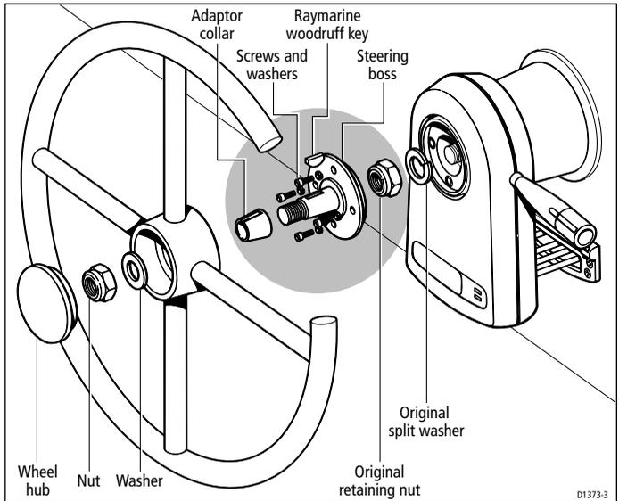
Fitting the SportPilot to 1 inch steering shaft
