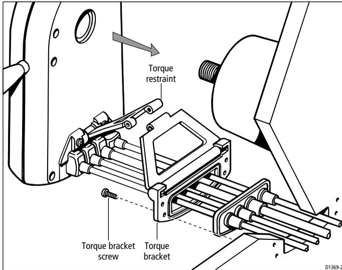
5. Assemble the SportPilot to the steering shaft.
