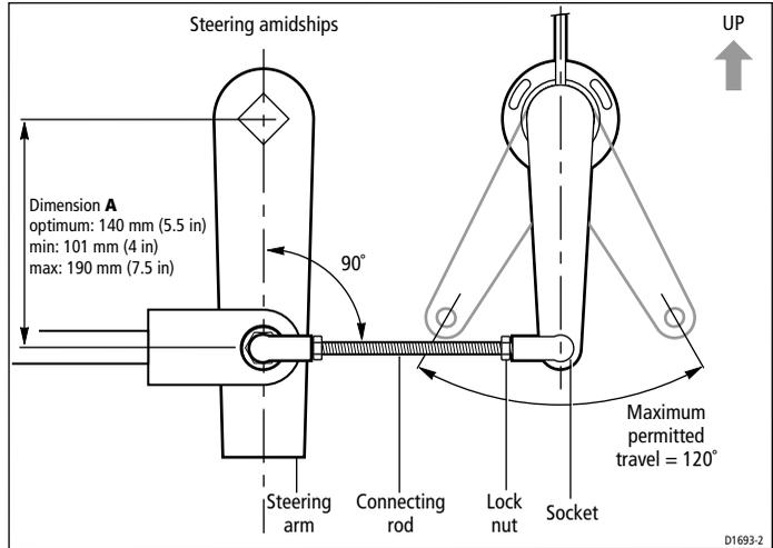
**Single drive system with vertical steering arm**
