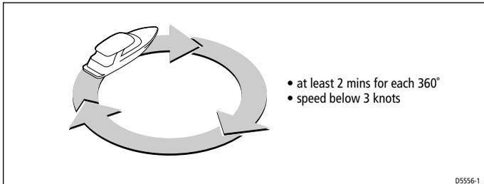
4. Keep turning your boat in circles until the SportPilot indicates that compass linearization is complete by:
