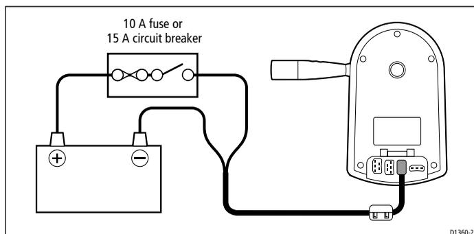
1. Connect the brown wire to the positive (12 V) terminal and the blue wire to the negative (0 V) terminal.
