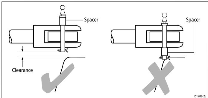
**Note:** The plastic spacer must be used to lift the pin so it does not foul on the steering system. If necessary, you can shorten the sleeve.
