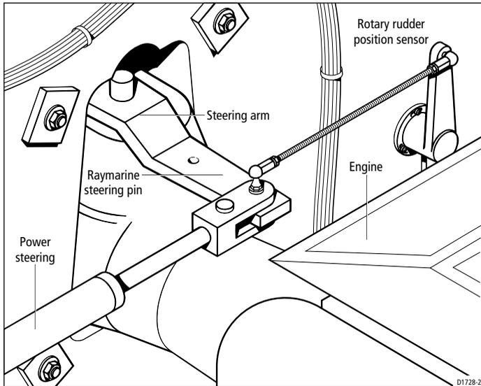
Typical installation – sensor connected to horizontal steering arm
