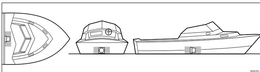
**Note:** To check if the intended mounting location is free from magnetic influence, tape a handheld compass to the chosen location, then turn the boat through 360°. The readings on the handheld compass and your boat's main steering compass (if accurately aligned) should not differ by more than 10° at any heading.
