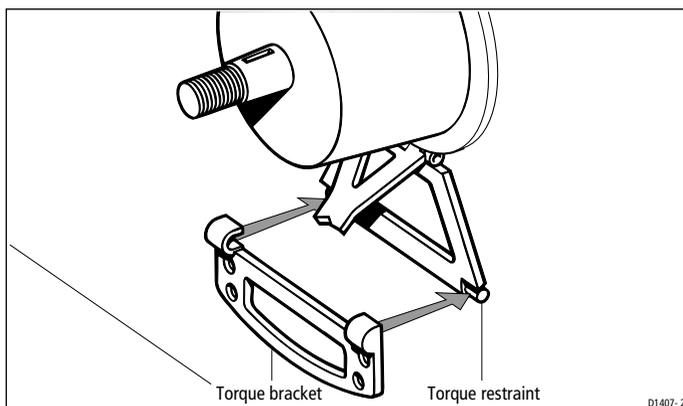
9. Make sure that the lower edge of the torque bracket is level with the bottom of the SportPilot.
