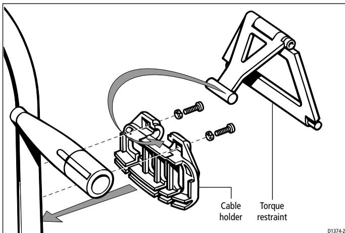
5. Temporarily assemble the cable holder to the SportPilot using the screws and washers.
