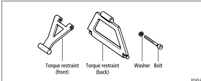
**Note:** *The torque restraint will not operate properly if the front and back are not assembled correctly. Therefore, once you have assembled the component parts, close the torque restraint as far as it will go. If you have assembled it correctly, the front will lay flat against the back.*
