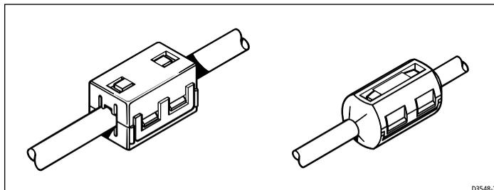
During installation you should position these ferrites as close as possible to the SportPilot, just behind the bulkhead. You may need to remove the ferrites during installation. If you do so, you **MUST** reassemble them around the cable when installation is complete.
